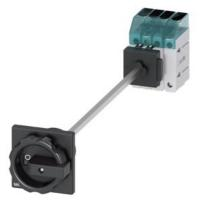
Load disconnector 3LD3, Iu 40 A Main switch 3-pole + N Rated operating capacity at AC-23 A at 400 V 18.5 kW floor mounting Basic switch with door coupling Central hole mounting 22.5mm Rotating drive black 66 x 66 mm
