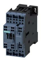
power contactor, AC-3 9 A, 4 kW / 400 V 1 NO + 1 NC, 24 V DC with plugged-in diode combination, 3-pole, Size S0, Spring-type terminal
