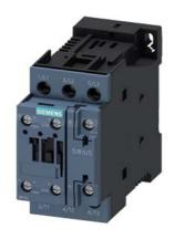
power contactor, AC-3 12 A, 5.5 kW / 400 V 1 NO + 1 NC, 24 V DC communication-capable, 3-pole Size S0, screw terminal
