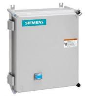
Non-reversing motor starter, Size 1, Single phase full voltage, Solid-state overload relay, OLR amp range 3-12A, 208VAC 60Hz coil, Non-combination type, Enclosure type 4X fiberglass, Water/dust tight noncorrosive, Standard width enclosure
