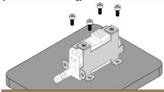
2pcs of M3.0  $\times$  8 Bolts are for Bracket plate. Apply 4pcs of proper M3.0 screws at your end according to your condition.
