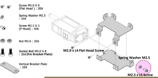
Make sure to use M2.5 spring washer to prevent damage.
