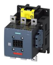
Power contactor, AC-3 265 A, 132 kW / 400 V Coil AC 50/60 Hz and DC 96-127 V x (0.8-1.1) F-SPS input 24 V DC 3-pole size S10 Auxiliary contacts 2 NO + 2 NC permanently mounted Main circuit: Busbar Control and auxiliary circuit: Screw terminal
