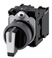
Selector switch, illuminable, 22 mm, round, plastic with metal front ring, white, selector switch, short, 3 switch positions I>O<II, momentary contact type, actuating angle  $2x45^{\circ}$ , 10:30h/12h/13:30h, with holder, 1 NO, 1 NO, screw terminal, with laser labeling, inscription or symbol Customer-specific selection with SIRIUS ACT configurator (CIN)
