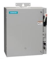
Pump control panel, Size 1, Three phase full voltage, Solid-state overload relay, OLR amp range 3-12A, 208VAC 60Hz coil, Standard type contactor, 10A circuit breaker, HOA Sel Sw. <(>&<)> Start P.B., Enclosure NEMA type 3/3R, Weather proof outdoor use
