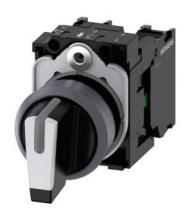
Selector switch, illuminable, 22 mm, round, plastic with metal front ring, white, selector switch, short, 3 switch positions I-O-II, latching, actuating angle  $2x45^{\circ}$ , 10:30h/12h/13:30h, with holder, 1 NO, 1 NO, screw terminal, Z=20-unit packaging
