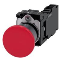
Mushroom pushbutton, 22 mm, round, plastic with metal front ring, red, 40mm, latching, pull-to-unlatch mechanism, with holder, 1 NO+1 NC, screw terminal, with laser labeling, upper case and lower case, always upper case at the beginning of the word
