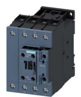
Power contactor, AC-3 40 A, 18.5 kW / 400 V 2 NO + 2 NC 220 V/240 V AC, 50/60 Hz 4-pole size S2 screw terminals 1 NO + 1 NC integrated
