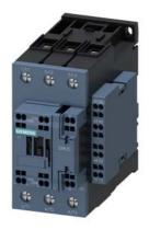
power contactor, AC-3 40 A, 18.5 kW / 400 V 2 NO + 2 NC, 230 V AC 60 Hz, 3-pole, Size S2, Spring-type terminal lateral auxiliary switch block
