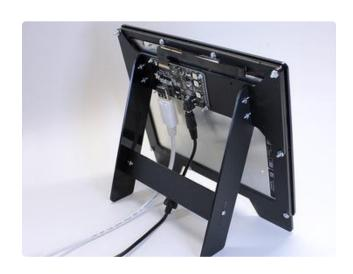
Stand the screen up and remove the tape pieces (if used) from the front bezel. Give it a very gentle tap on the desk to make sure everything's seated, then work around the perimeter tightening these screws. Just snug them down a little...don't go crazy or you'll crack the plastic.
