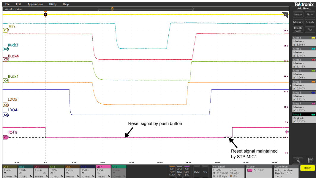
Figure 13. Reset sequence for STPMIC1A configuration
