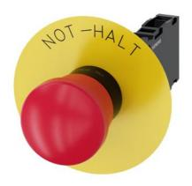
EMERGENCY STOP mushroom-type actuator, 22 mm, round, plastic, red, 40 mm, positive latching, according to EN ISO 13850, pull-to-unlatch mechanism, with yellow backing plate, inscription: NOT-HALT, with holder, 1 NO+1 NC, screw terminal, Z=20-unit packaging
