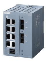
SCALANCE XB108-2 unmanaged IE switch, 8x 10/100 Mbit/s Ports, 2x 100 Mbit/s multimode SC, for setting up small star and line topologies; LED diagnostics,IP20, redundant power supply, 24 V AC/DC Manual available as a download .
