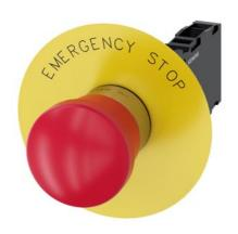
EMERGENCY STOP mushroom pushbutton, 22 mm, round, metal, shiny, red, 40 mm, positive latching, acc. to EN ISO 13850, pull-to-unlatch mechanism, with yellow backing plate, inscription: EMERGENCY STOP, with holder, 1 NO+1 NC, screw terminal
