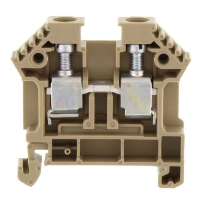
Feed-through terminal, Screw connection, Mounting type: Mounting rail TS 35/7.5, Rated cross-section: 10 mm², Width: 8 mm, Colour: Beige
