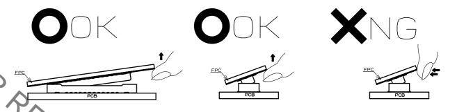
FPC IS NOT RIGID, THE CONNECTOR CAN BE BROKEN. PLEASE CHECK THE ACTION OF THE FPC TO BE USED REPEATEDLY AT THE TIME OF TRIAL PRODUCTION. BE CAREFUL TO UN-MATE THEM FROM THE PITCH DIRECTION. THE CORNER CAN ALSO RISK TO PUTTING STRESS ON CONTACTS.
