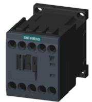
Power contactor, AC-3 16 A, 7.5 kW / 400 V 1 NC, 400 V AC, 50 Hz 400-440 V, 60Hz, 3-pole Size S00, screw terminals
