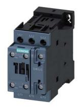
Power contactor, AC-3 17 A, 7.5 kW / 400 V 1 NO + 1 NC, 24 V DC with varistor 3-pole, Size S0, screw terminal
