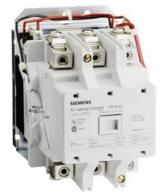
Mechanically held lighting contactor, Contactor amp rating 100A, 0 N.C. / 2 N.O. poles, 440VAC 50HZ/480VAC 60HZ coil, Non-combination type, Enclosure NEMA type (open), No enclosure
