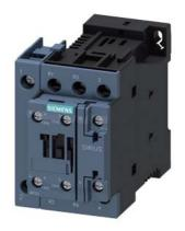
Power contactor, AC-3 25 A, 11 kW / 400 V 2 NO + 2 NC 110 V DC, 50 Hz 4-pole size S0 screw terminals 1 NO + 1 NC integrated
