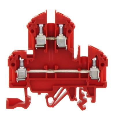
Double-level terminal, Screw connection, Mounting type:Mounting rail TS 35/7.5 and TS 32, Rated cross-section: 4 mm², Width: 6 mm, Colour: Red
