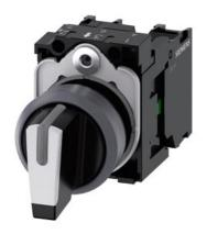
Selector switch, illuminable, 22 mm, round, plastic with metal front ring, white, selector switch, short, 3 switch positions I>O<II, momentary contact type, actuating angle 2x45°, 10:30h/12h/13:30h, with holder, 1 NO, 1 NO, screw terminal
