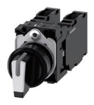
Selector switch, illuminable, 22 mm, round, plastic, white, selector switch, short, 3 switch positions I>O<II, momentary contact type, 10:30h/12h/13:30h, with holder, 2 x 1 NO+1 NC, screw terminal, Z=20-unit packaging
