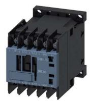
Power contactor, AC-3 9 A, 4 kW / 400 V 1 NO, 200 V AC, 50 Hz 200-220 V, 60 Hz, 3-pole, Size S00, ring cable lug connection
