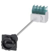
SENTRON, Switch disconnector 3LD, main switch, 4-pole, lu: 32 A, Operating power / at AC-23 A at 400 V: 11.5 kW, floor mounting with door coupling, rotary operating mechanism, black, 4-hole mounting of the handle
