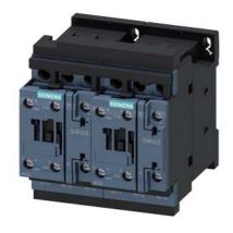
Reversing contactor assembly AC-3,11 kW/400 V,AC110V,50/60Hz 3-pole, Size S0 screw terminal electrical and mechanical Interlock 2 NO integrated
