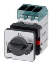
Load disconnector 3LD3, lu 16 A Main switch 3-pole Rated operating capacity at AC-23 A at 400V 7.5kW Front plate mounting Basic switch with Central hole mounting 22.5mm Toggle drive black 48x48 mm
