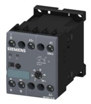
Timing relay, electronic ansprechverzögert 1 change-over contact 24 V AC/DC, 200 to 240 V AC at 50/60 Hz AC 0.05 s to 100 h Overall width 45 mm screw terminal
