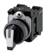
Selector switch, illuminable, 22 mm, round, plastic with metal front ring, white, selector switch, short, 3 switch positions I>O<II, momentary contact type, actuating angle 2x45°, 10:30h/12h/13:30h, with holder, 1 NO, 1 NO, spring-type terminal, Z=20-unit packaging
