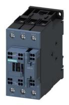
Traction contactor, AC-3 65 A, 30 kW / 400 V 1 NO + 1 NC 110 V DC, 0.7-1.25\* Us with varistor 3-pole, size S2 Spring-type terminals
