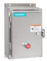
Non-reversing motor starter, Size 2, Three phase full voltage, Solid-state overload relay, OLR amp range 13-52A, Non-combination type, Encl. type 4X 304 S. Steel, Water/dust tight noncorrosive, Standard width enclosure
