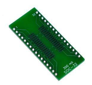
SOIC-32, SOP-32, SMD to DIP Adapter
