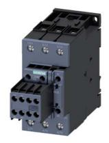
Power contactor, AC-3 80 A, 37 kW / 400 V 2 NO + 2 NC, 42 V AC, 50 Hz 3-pole, size S2 screw terminals
