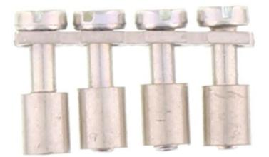
Cross-connector, No. of poles: 4, Mounting type: Can be screwed on, Width: 19.3 mm, Rated cross-section: 2.5 mm<sup>2</sup>, Colour: natural
