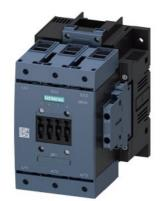
power contactor, AC-3 115 A, 55 kW / 400 V AC (50-60 Hz) / DC operation 110-127 V AC/DC auxiliary contacts 2 NO + 2 NC 3-pole, frame size S6 with box terminals drive: conventional screw terminal
