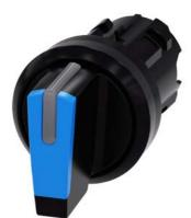
Selector switch, illuminable, 22 mm, round, plastic, blue, selector switch, short, 3 switch positions I-O<II, left latching, right momentary contact type, actuating angle  $2x45^{\circ}$ , 10:30h/12h/13:30h
