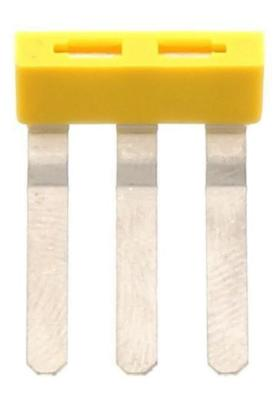
External insulated cross-connector, No. of poles: 3, Mounting type: Plug in, Width: 16.9 mm, Rated current: 27 A; Colour: Yellow
