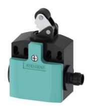
Position switch Plastic enclosure, 50 mm Device connection 2 x (M20 x 1.5) 1 NO/2 NC quick action contacts with M12 connector, 4-pole on the right, 2 NC connected Pin assignment: Pin1=21, Pin2=22 Pin3=31, Pin4=32 max. 250 V and 4 A Roller lever with plastic roller 13 mm
