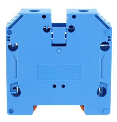
Feed-through terminal, Screw connection, Mounting type: Mounting rail TS 35/7.5, Rated cross-section: 50 mm², Width: 18.5 mm, Colour: Blue
