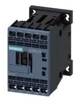
Power contactor, AC-3 7 A, 3 kW / 400 V 1 NC, 60 V DC 3-pole, Size S00 Spring-type terminal
