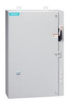
Non-reversing motor starter, Size 3, Three phase full voltage, Solid-state overload relay, OLR amp range 25-100A, 24VAC 50-60Hz coil, Combination type, 100A fusible disconnect, 100A/250V fuse clip, Enclosure NEMA type 4/12, Water/dust tight for outdoors, Standard width enclosure
