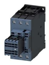
traction contactor, AC-3 51 A, 22 kW / 400 V 2 NO + 2 NC 72 V DC, 0.7-1.25\* US, with varistor, 3-pole, size S2, spring-loaded terminal
