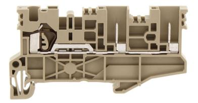
Feed-through terminal, Tension-spring connection, Mounting type: Mounting rail TS 35/7.5, Rated cross-section: 2.5 mm<sup>2</sup>, Width: 5.1 mm, Colour: Beige
