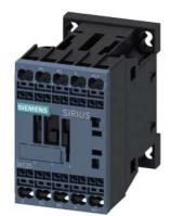
Power contactor, AC-3 9 A, 4 kW / 400 V 2 NO + 2 NC 220 V DC 4-pole Size S00 Spring-type terminals
