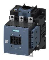
power contactor, AC-3 185 A, 90 kW / 400 V AC (50-60 Hz) / DC operation 200-277 V AC/DC auxiliary contacts 2 NO + 2 NC solid-state-compatible, 3-pole, frame size S6, busbar connections drive: electronic with PLC interface 24 V DC
