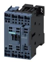
Contactor, AC-1, 40 A/400 V/40 °C, S0, 4-pole, 220 V DC, 1 NO+1 NC, Spring-type terminal
