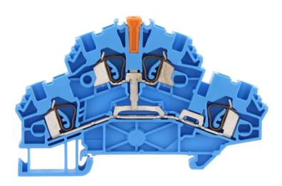
Double-level terminal, Tension-spring connection, Mounting type: Mounting rail TS 35/7.5, Rated cross-section: 2.5 mm², Width: 5.1 mm, Colour: Blue
